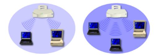
**Single AP Bridge** Another possible AirConnect topology is a single AP bridging an Ethernet and wireless network. As shown in the next figure, the AP, wired to a network server or LAN through an Ethernet cable, serves as a network node and provides the link between the server and the wireless clients. The wireless clients can move freely throughout the coverage area of the AP while remaining connected to the server.
